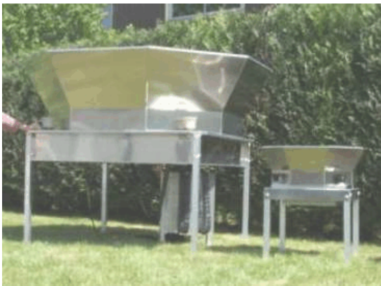
Figure 8. SODAR model PA5 (1.8x1.8 meter footprint) has a range 15 – 5000 meter (average altitude under typical conditions 3500 m); frequency 800 Hz, and model PA1 (0.65x0.65 meter footprint) has a range 15 – 2000 meters. (average altitude under typical conditions 1300 m); frequency
